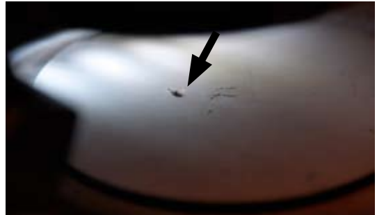
Figure 4. Small light dot shining on a Polygala seed, indicating field of view for positioning your material.
