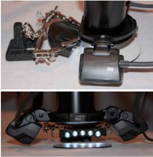
Figure 3. Electrical 'crabs' arms' stand holding LED focussing light. Top: Side view. Bottom: Front view.
